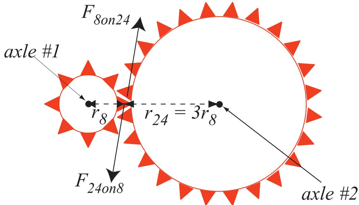
Since torque =  $r \times F$ , the torque about axle #2 is three times greater than the torque about axle #1; the gear train acts as a **“torque amplifier”**.
