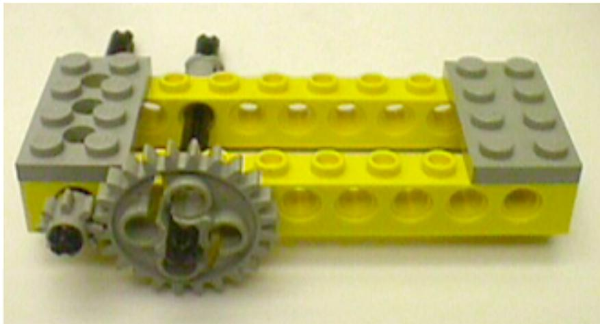
Try rotating the shaft with the small gear with your fingers. Note that the relative rate of rotation of the two axles is different, by a factor of three, which is equal to the ratio of number of teeth on the gears (24:8).
