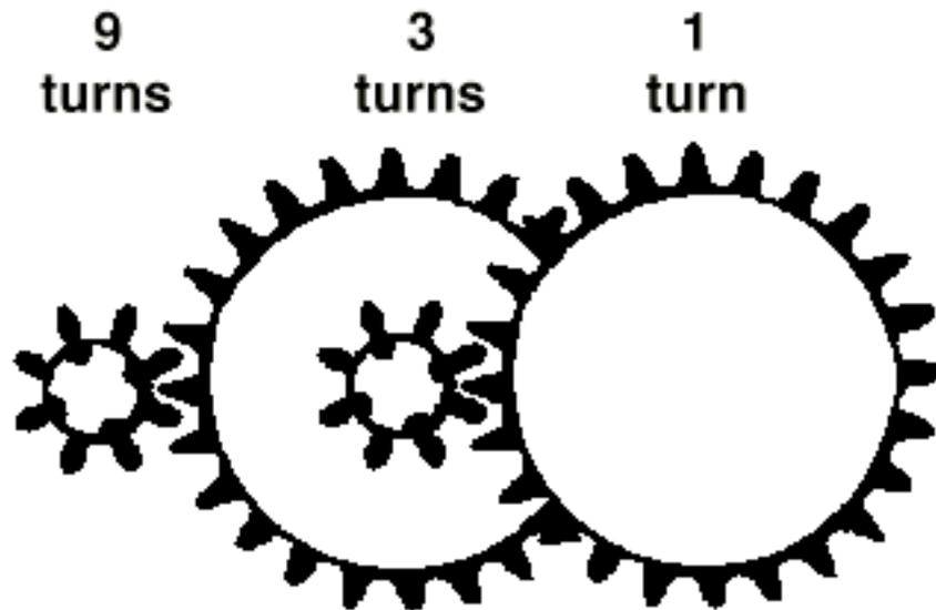
By “ganging together” – or multiplying – two 3-to-1 gear reductions, a 9-to-1 output reduction can be achieved. The key is to use intermediary shafts that hold both a large input gear (e.g. a 24-tooth) and a small output gear (e.g. an 8-tooth).
