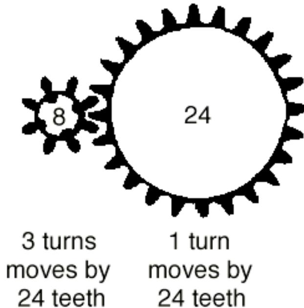
When the 8-tooth gear rotates 3 times, it advances the meshed gear by a total of 24 teeth. Since the meshed gear has a total, it rotates exactly once. (We say this configuration has a **3:1 gear ratio**.) Thus the 24-tooth gear rotates *three times slower* than the 8-tooth gear.
