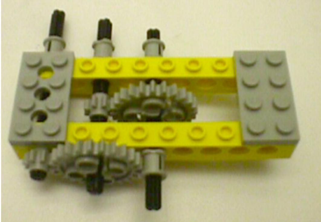
So now the torque at the “output shaft” is 9 times the torque provided on the left (“input”) axle. The output shaft will of course spin 9 times slower than the input shaft, but it will be much harder to stall!
