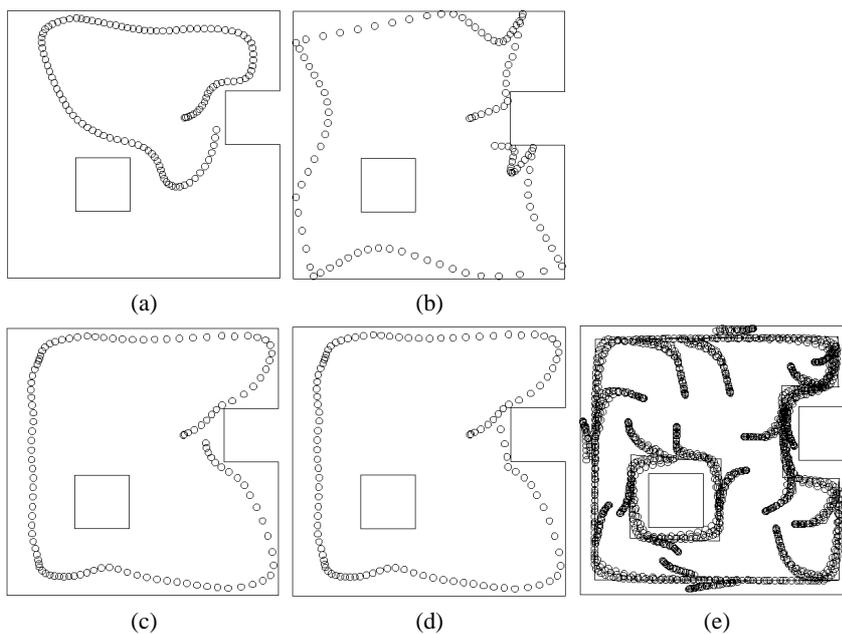
**Fig. 3.** Experimental results obtained with a RIB having the following subsets of rules: a) obstacle-avoidance, motion and wall-following rules; b) obstacle-avoidance, motion and wall-approaching rules, c) obstacle-avoidance, motion, wall-approaching and wall-following rules, d) as in c) plus corner following rule, e) the training set for the wall-following neural net. (S=start)
