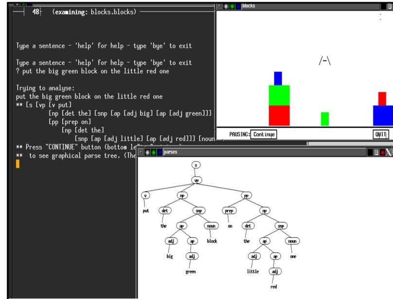
**Above:** how the machine understands a command “put the big green block on the little red one” -- showing the structure of the sentence diagrammatically. Having understood, it then makes a plan to achieve the goal. (The /-\ represents a hand!)
