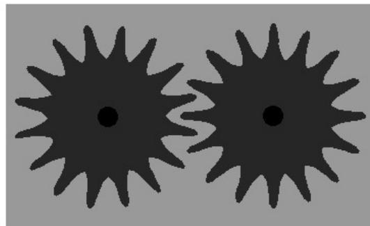
It is also possible to use the physical gears to do a thought experiment! This involves considering the details of what happens when one wheel is rotated about a fixed axis, and how it applies a force to the other wheel (through the cogs that are currently meshed) and how the rigidity and impenetrability constrain the effects of motion of a cog, and also how the geometry ensures that there is always at least one cog of the wheel being turned that is in contact with a cog on the
