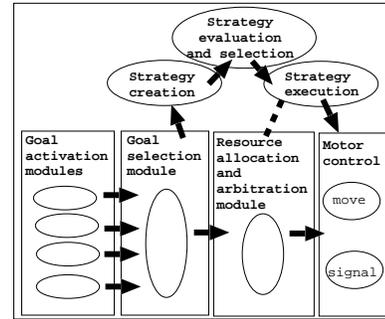
Figure 4: The Hybrid Design **HAR**. Deliberative mechanisms provide a secondary route to action, activated as a result of interrupts to reactive selection and arbitration and imposing different actions. The dashed line represents an inhibitory interaction initiated by the Strategy execution module.
