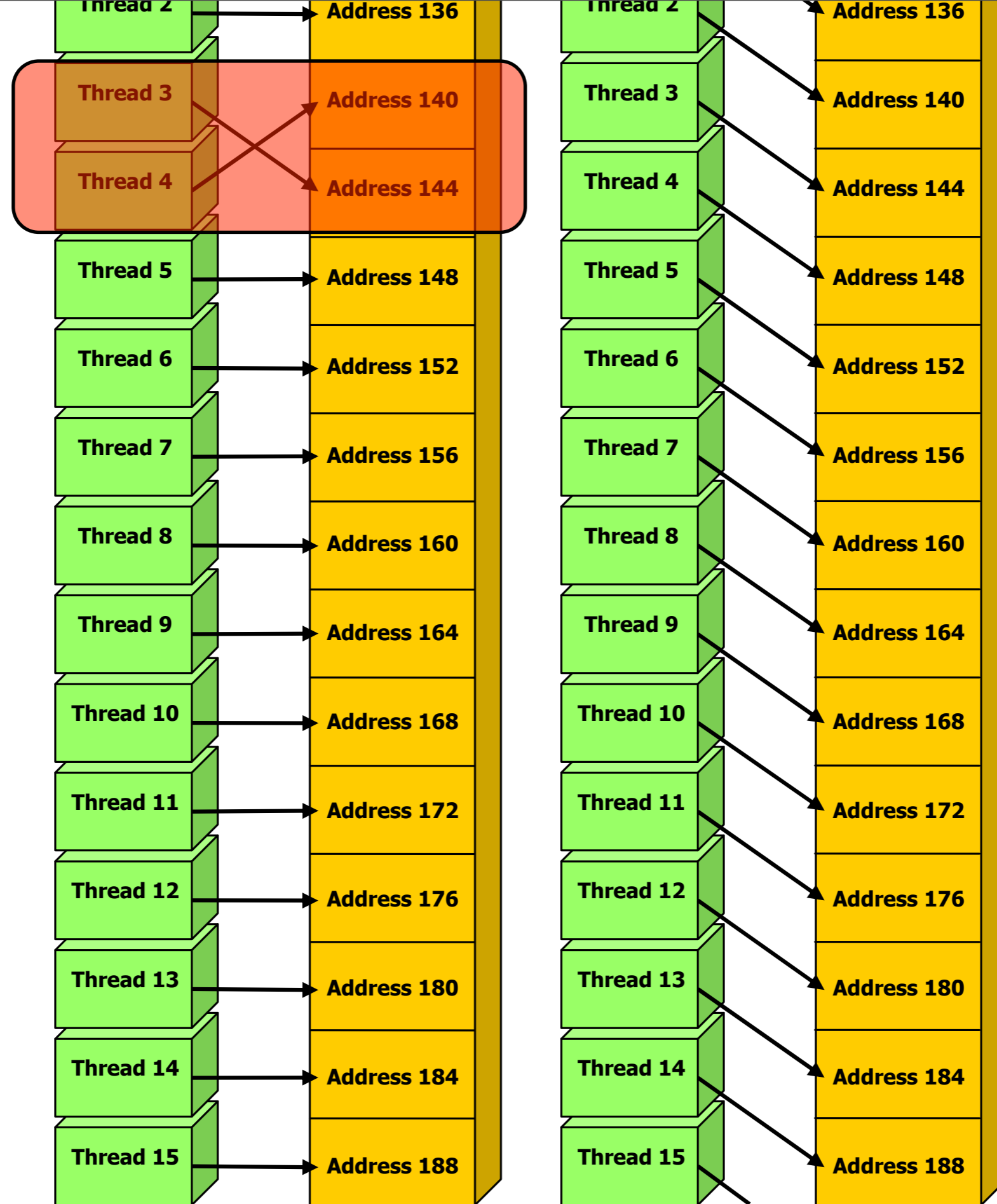
Left: non-sequential float memory access, resulting in 16 memory transactions.
