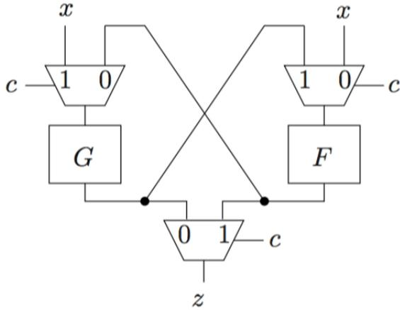
Fig. 1. Combinational circuit with (false) feedback ([10, Fig. 1])
