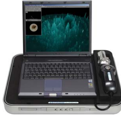
Figure 5. The SIAScope II – a commercial device for skin imaging and computation of SIAGraphs. Images are acquired using a handset (at the bottom right of the case) connected to a laptop computer. The image interpretation is implemented on the computer and SIAGraphs are displayed on its screen.
