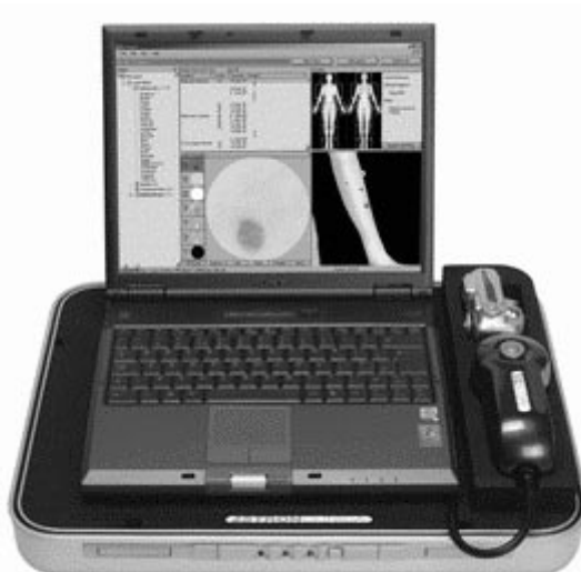
Fig. 4. SIAscope – a certified commercial device developed using the model of skin colouration described in this paper.
