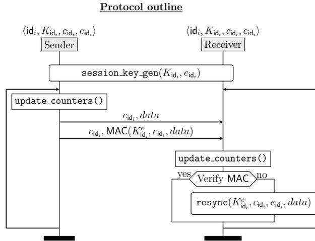
**Figure 4.** Communication between sender  $S$  and receiver  $R$  for message with identifier  $id_i$  – LEIA protocol outline: first, the session keys are generated by both participants; then,  $S$  can send authenticated message to  $R$ ;  $R$  verifies the MAC of the received message; if the verification fails, the resynchronisation is initialised, otherwise, the message is accepted.
