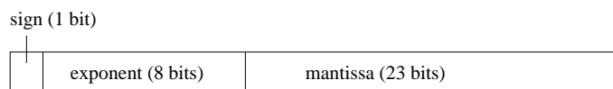
Figure 4.1: The mantissa in a 32-bit ‘single’ precision is represented by 23 bits and the exponent by 8 bits. The remaining bit is used for the sign.
