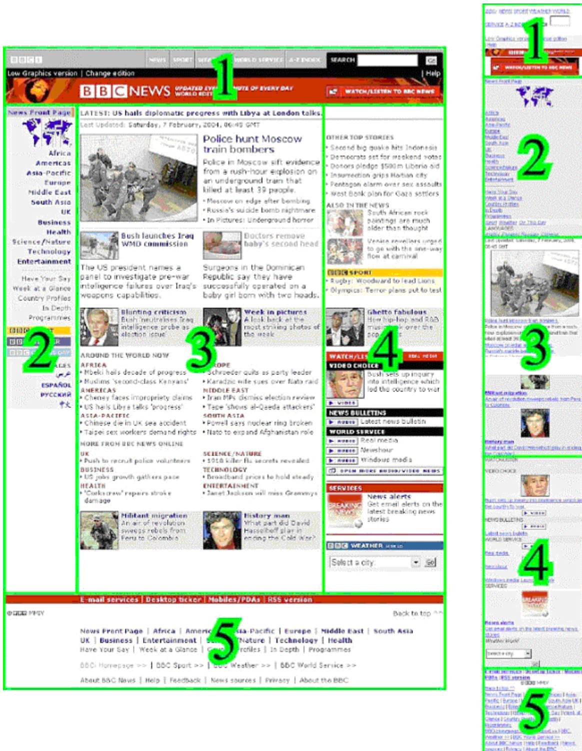
Figure 1: Opera browser renders HTML content in the order in which it is defined
