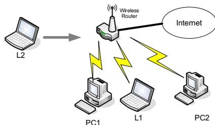
**Figure 2: Wireless Router used in a PAN**
