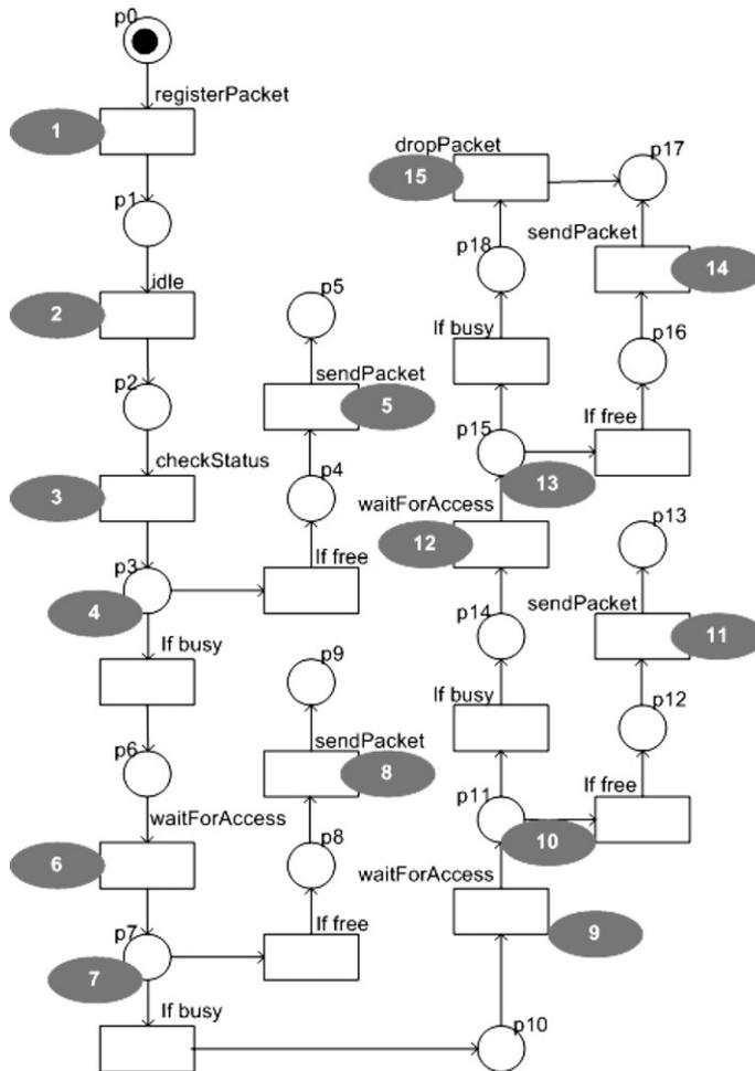
Fig. 10. Petri Net for a station in PAN.
