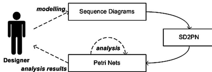
Fig. 1. SD2PN model transformation framework.
