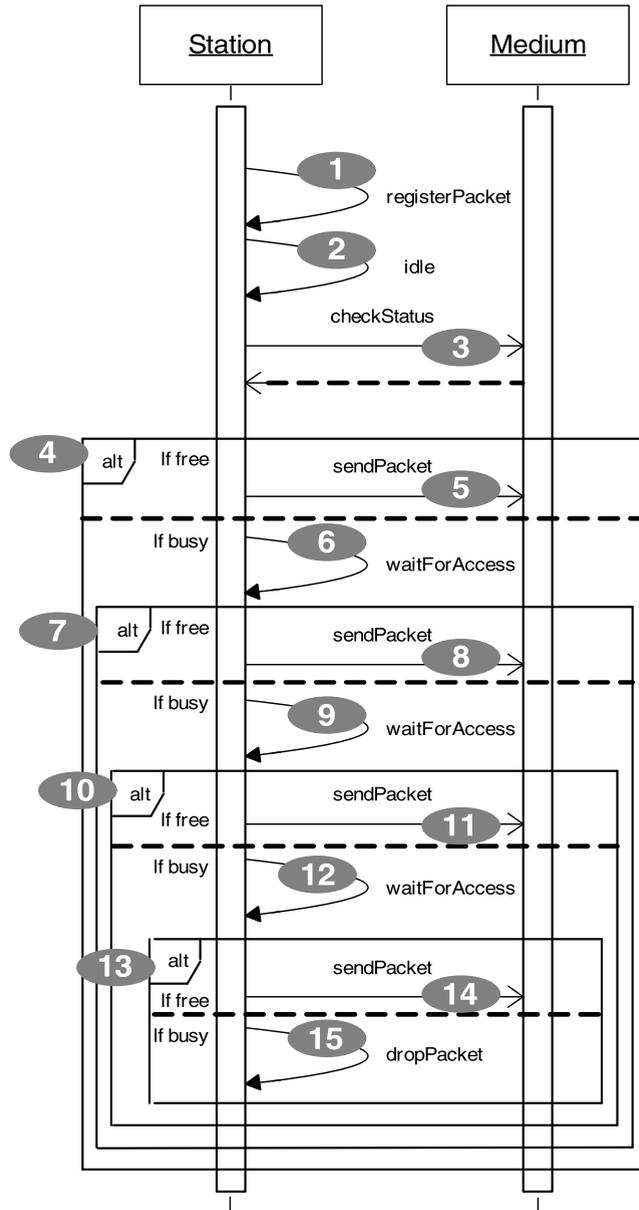
Fig. 6. Sequence Diagram for a station in PAN.
