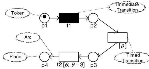
Fig. 15. Example of a Timed Petri Net.
