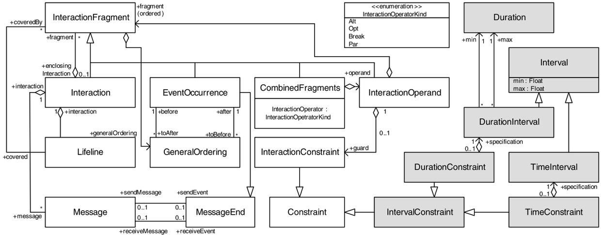
Fig. 12. Sequence Diagram metamodel augmented with timeliness properties.
