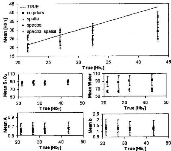
Fig. 3. Mean reconstructed values of  $[\text{Hb}_T](\mu\text{M})$ ,  $S_t\text{O}_2$  (%), water (%),  $A$ , and  $b$ , in the region of the inclusion using four algorithms. When the blood concentration is high, the best results are achieved by combining spectral and spatial priors. As expected,  $S_t\text{O}_2$ , water,  $A$ , and  $b$  within the cavity remain constant.
