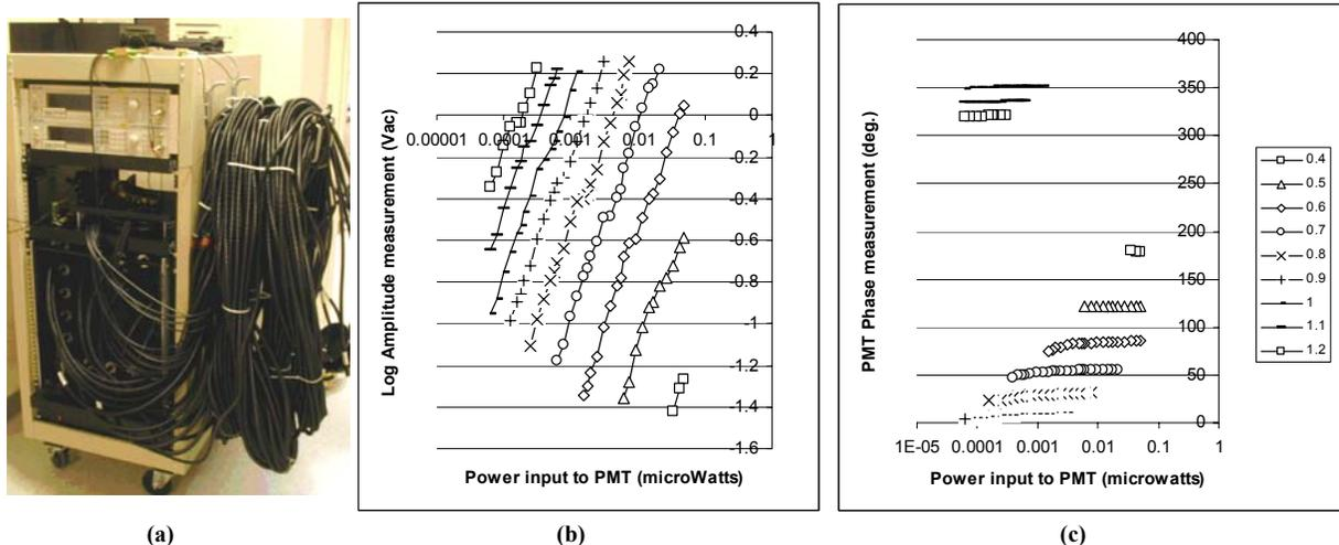
**Figure 1.** (a) The mobile NIR tomography system with long fibers for measurement inside the MRI. Graphs (b) and (c) show measurements used to calibrate a representative PMT. In (b) the Log Amplitude response is shown to be linear with input log of optical power. The phase response does not change significantly with input power changes, as long as the amplitude is within a linear range, with adequate signal to noise ratio.
