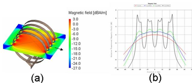
FIG. 4. (Color online) (a) Relative transversal magnetic field of the solenoid coil. The isocenter is set to 0 dB and the arrow shows the  $B_0$  direction. (b) Sensitivity profiles along the coil axis (perpendicular to the main field  $B_0$ ) for different distances from the isocenter.
