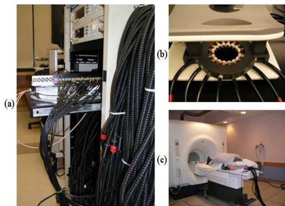
**Figure 1.** Photograph of the portable cart housing the NIR light generation and detection hardware. The cart stands outside of the RF shielded MR chamber, and optical fibers extend 13 meters to the MRI patient bed.
