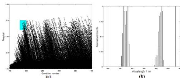
**Figure 1.** (a) Scatter plot of the residual and condition number calculated for 3 chromophores, hemoglobin, deoxy-hemoglobin and water. (b) Histogram of optimized wavelength.
