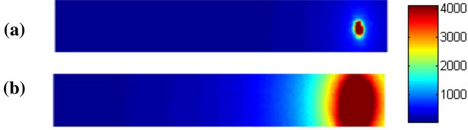
**Figure 2:** A pair of images illustrating what is known as CCD blooming. The approximate size of the laser beam is an ellipse of size 1mm x 1.5 (a). When the camera's integration time is increased the charge overflows from pixel wells in the position of the laser spot and into the neighboring wells (b). In this system blooming artifacts in the data make imaging large fluorescent targets difficult.
