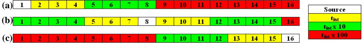
**Figure 3:** Examples of the optimal data acquisition scheme which involved reading the data out in three distinct bins. Here, the white rectangle represents the position of the active laser source, and the yellow, green, and red blocks represent integration time increases of 1x, 10x, and 100x respectively. This approach was necessary to maintain a suitable SNR at the detectors located far from the source. A  $t_{\text{int}}$  of 50ms was used in this work.
