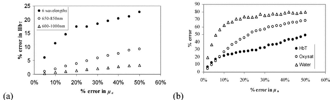
**Figure 2(a)** The percent error in the calculated total hemoglobin value is estimated based upon spectral fitting with random errors assumed in the absorption coefficient. Results show how the error would change when different numbers of wavelengths are used in the measurements. In (b) the same error propagation calculation is shown with a bias error model demonstrating how this error is amplified for the same error in absorption.
