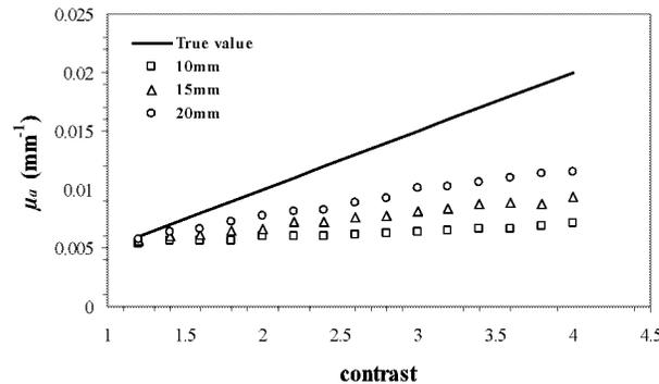
**Figure 1.** Reconstructed absorption coefficient for different sized inclusions, as a function of the contrast relative to the background absorption. These are simulated data with region of interest values taken from the final images.
