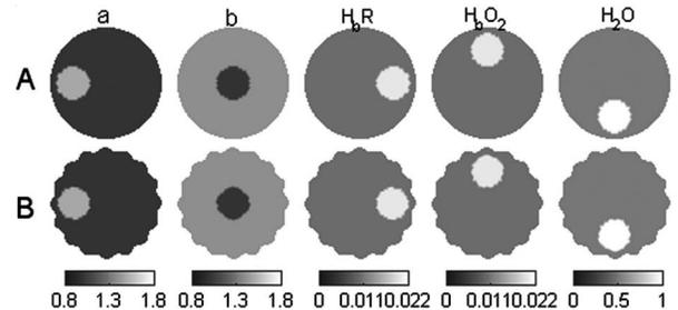
Fig. 2. A, Target phantom with five distinct inclusions (diameter=27 mm). Each column corresponds to the particular parameter. B, Target phantom for a simulation where an irregular boundary was considered.
