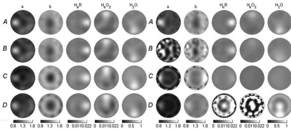
Fig. 3. A–D, Reconstructed images of simulations for both SDIR (left) and DCSR (right), with A, images having no data errors; B, 5% randomly distributed coupling errors; C, boundary reflection coefficient modeling error; D, reconstructing data taken from a distorted boundary shape.
