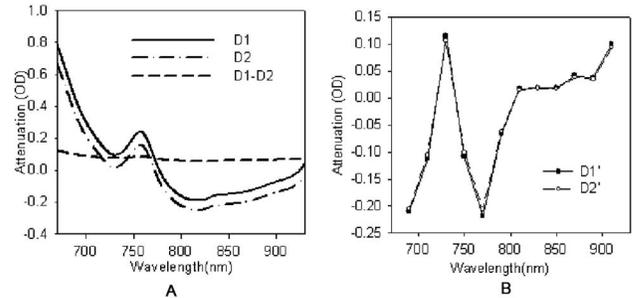
Fig. 1. A, Experiment geometry and source–detector fiber configuration. B, Measured attenuation spectra at D1, D2 and their difference. C, First-order finite difference spectra of D1 and D2 with a 20 nm separation.
