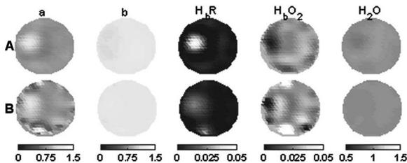
Fig. 4. Reconstructed images of a liquid phantom for both A, SDIR and B, DCSR. The background was 0.03 mM fully oxygenated blood with 1% Intralipid and the inclusion contained in a thin and clear straw was 0.09 mM fully deoxygenated blood with 2% Intralipid.
