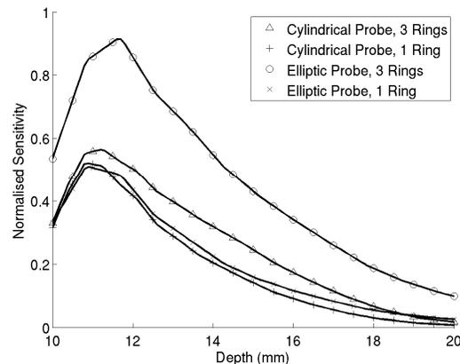
**Figure 3.** Cross sectional normalized sensitivity profile for each probe design as a function of depth
