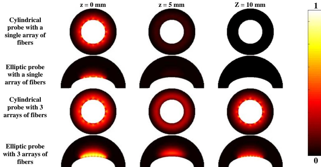
**Figure 2.** The normalized sensitivity of each probe design and fiber arrangement strategy. The images presented are coronal cross-sections of the 3D model at different sections. Note that for the cylindrical case the depth of tissue modeled as surrounding the probe is set at 10 mm, where as in the elliptic case the depth of tissue modeled as surrounding the probe is set at 20 mm in the short axis and 10 mm in the long axis.
