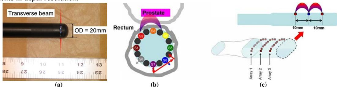
**Figure 1.** (a) The cylindrical transrectal probe and (b) 2D cross-section showing the source and detector arrangements. (c) proposed elliptical probe design consisting of either a single layer of source and detectors in a single array, or two array of detectors with a single array of sources in between.
