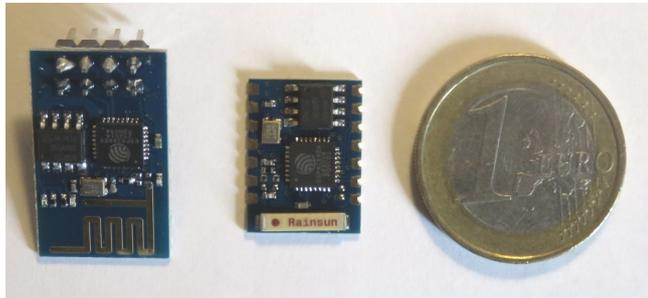
**Fig. 1.** Different ESP modules, Euro coin for scale.
