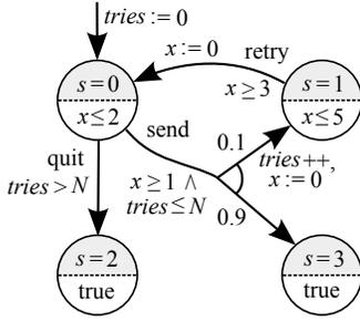
Fig. 1. A simple PTA, with clock  $x$  and integer variable  $tries$ , modelling the attempted message transmission of a message over an unreliable communication channel.
